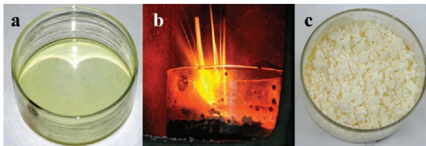
FIGURE 1. (a) Aqueous solution of ceric ammonium nitrate, Pd nitrate, and oxalylidihydrazide, (b) the solution burning with a flame, and (c) the oxide product.
